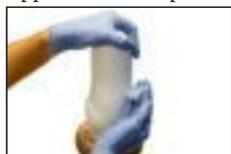
Take an amount of 633F50 Silicone Grease adequate for the model and apply it evenly and thinly to the model.
