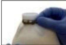
Using the pre-formed plastaband, isolate the corresponding areas of the objects that will be included in the laminate (e.g. screw heads, bare threads, joint surfaces).
