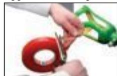
Use 634A58 Isopropyl Alcohol to clean the surfaces that are to be bonded (here the inner socket and the frame). Cut 633D5 Double Sided Adhesive Tape to the required length.
