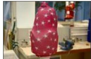
Turn the decor fabric so that the design faces outwards, and then pull it over the socket model. Place the seam in a less conspicuous position on the socket (e.g. medially).
