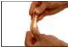
Stretch and fold both Pastasil components between your fingers several times until both components form a single-coloured mass.
