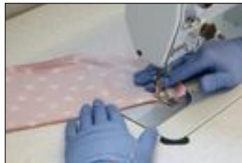
Tuck the decor fabric in within the marked contour and with a 5 mm reduction. Allow the distal seam to taper off. The seam can then only be seen on the medial side. Using a pair of scissors, cut to size along the outer side of the seam leaving a maximum of 2 mm of the decor fabric behind the seam.
