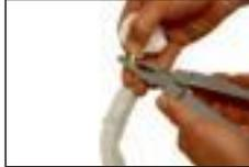
Pre-tension the 99B25 Residual Limb Sock, twist it and then secure it with combination pliers. Using a pair of scissors, cut off the end of the seam.
