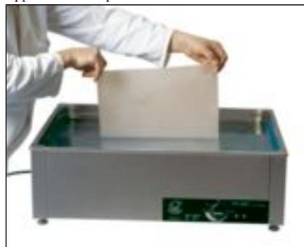
Place the pre-cut ThermoLyn Pedilon into warm water at approximately 60 °C/140 °F in the 759P1=220 water pan. The material becomes transparent when it reaches its moulding temperature. Remove the pre-cut material with a wooden spatula and allow the water to drip off.
