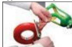
Use 634A58 Isopropyl Alcohol to clean the surfaces that are to be bonded (here the inner socket and the frame). Cut 633D5 Double Sided Adhesive Tape to the required length.
