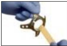
Prior to laminating, apply silicone grease to the objects that are to be isolated (e. g. thread of a screw, lamination dummy, adapter, orthotic joint). Attention: do not isolate those areas that are to create a bond with the lamination resin.
