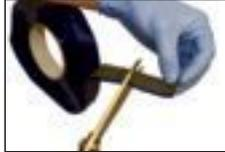
Cut 636K8 Plastaband to the required length.
