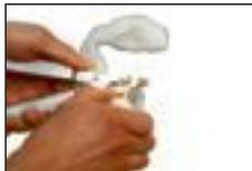
Using the flame of a cigarette lighter, weld the cut surface and then immediately smoothen the weld seam.
