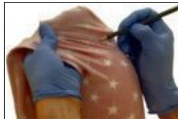
Pull the decor fabric around the socket model with the design facing inwards. Use your hand to pre-tension the decor fabric and, with the help of a pencil, transfer the socket contour. Do not use permanent markers, ball-point pens etc., because these could cause discolourations during the laminating process.
