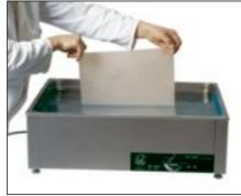
Place the pre-cut ThermoLyn Pedilon into warm water at approximately 60  $^{\circ}$ C/140  $^{\circ}$ F in the 759P1=220 water pan. The material becomes transparent when it reaches its moulding temperature. Remove the pre-cut material with a wooden spatula and allow the water to drip off.
