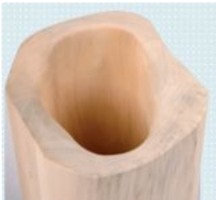
SF5P1=010 Smoothing the socket after copying
